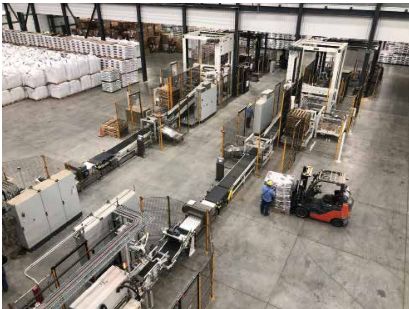
Diamond V contacted Concetti in 2018 to provide two new automated bagging, palletizing, and wrapping lines for their animal feed ingredients.
