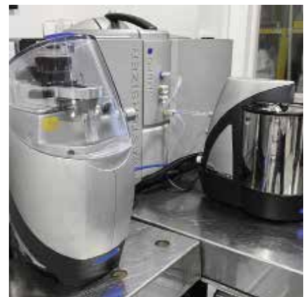
A laser diffraction unit is used to assess a powder's particle size.
