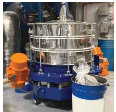
The high-energy sieving system separates powder using a strong vertical vibration.
