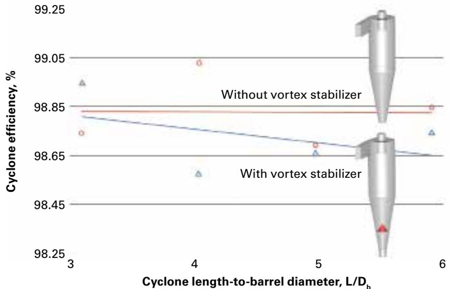
cyclones with the vortex stabilizer, the bed height in the dipleg was only 40 to 50 percent of the bed height for the cyclones without a vortex stabilizer. These results suggest that retrofitting a cyclone to include a vortex stabilizer can be readily accomplished, as modifications to an existing dipleg may not be needed.
