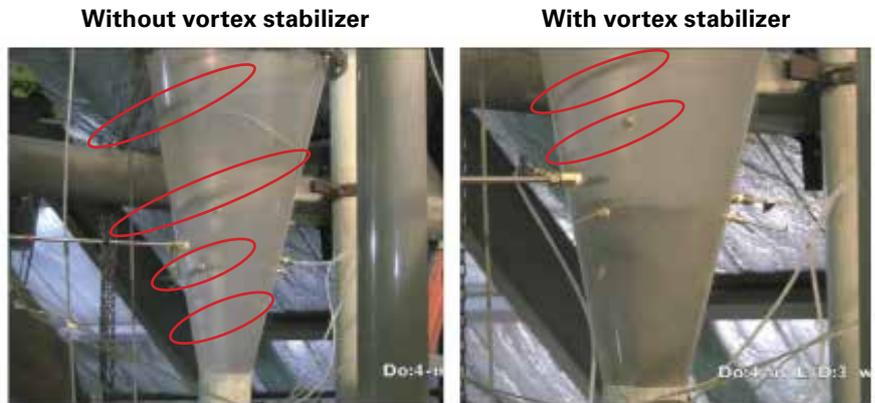
another way, a cyclone with a vortex stabilizer may be able to operate at a higher outlet gas velocity without suffering strong consequences from erosion in the lower cone region. Thus, increasing the outlet gas velocity could rectify the collection efficiency issue and may even exceed the cyclone's efficiency without the vortex stabilizer while
