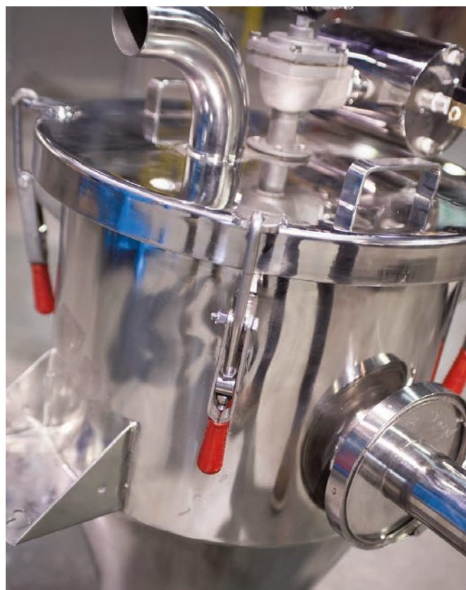
Vacuum transfer systems have virtually no moving parts and can gently transfer pharmaceutical ingredients using mass flow, preventing segregation.
