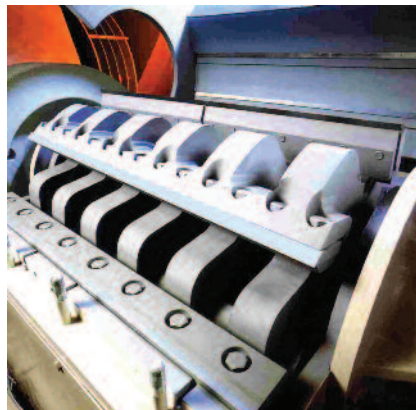
This knife mill has an operator-friendly design that provides easy access to the grinding chamber to simplify cleaning and wear parts replacement.
