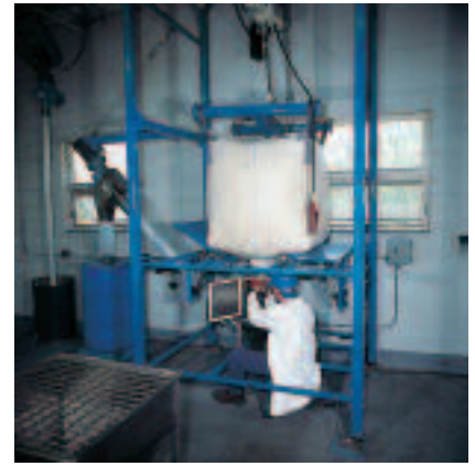
At the test center, AFC also conducts tests using the company’s bulk bag unloader.
