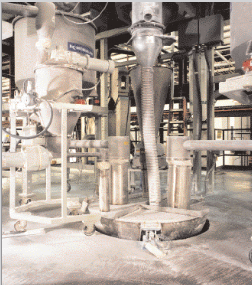
Modular feeders can be quickly reconfigured for dispensing ingredients with different handling characteristics.
