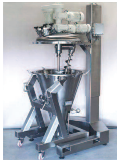
Conical screw mixer
