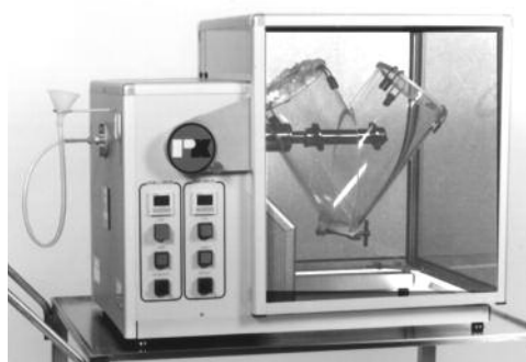
V-shaped blender (lab-size unit)
