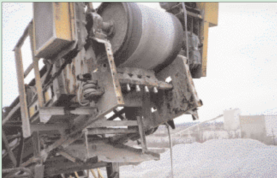
Here, on a belt conveyor carrying sand, a belt scraper mounted at the head pulley removes carryback from the top cover.
