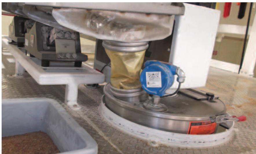
***The new flexible connector fitting between the vibratory screener’s discharge and auger feeder’s inlet easily snaps into place without tools and maintains a dust-tight seal during operation.***
