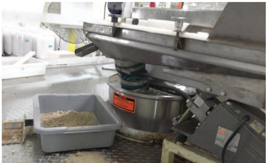
*A standard clamp-and-sleeve connector between the vibratory screener's discharge and auger feeder's inlet often allowed material to leak out onto the equipment, creating housekeeping and maintenance problems.*
