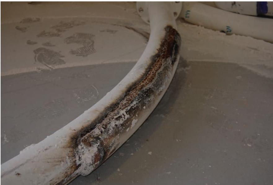
***The company had to remove this long-radius sweep elbow from the conveying line because the abrasive pebble lime wore a hole through its outer wall.***
