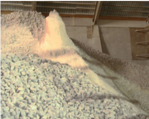
b. Angle-of-repose segregation in a stone pile
