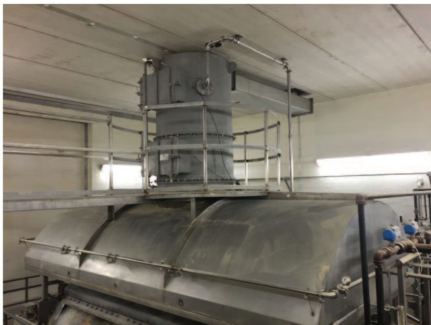
The Impinjet scrubber was custom-built to fit on top of Aveka's dryer to clean food flavor particles and dust flakes from the exhaust air.
