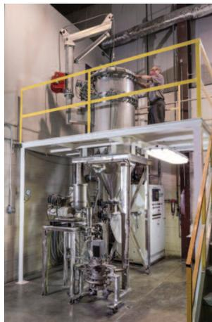
**A lab-sized fluidized-bed jet mill (bottom) is used for testing material grindability and throughput rates.**
