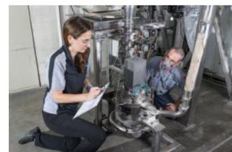
**A chemical engineer and mill operator examine a material after micronizing in a fluidized-bed jet mill.**
